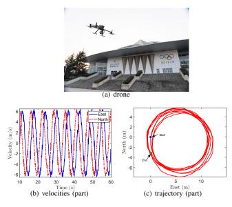
Fig. 2. Drone, its real-time velocities, and traveling trajectory, starting from 10s and ending at 60s (data credit: Competitive Robot Base, Northwestern Polytechnical University, Xi'An, China).
